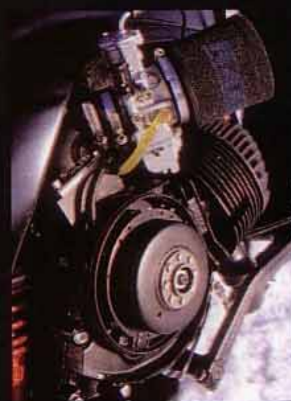
The Scooter & Service downdraught reedvalve conversion.
