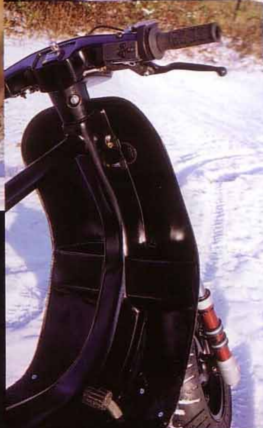
Modified legshields allow for movement of the telescopic fork top.
